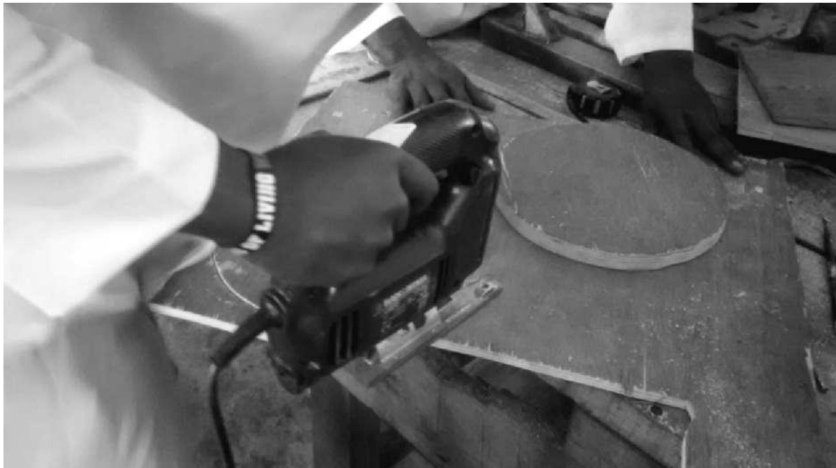
Fig. 1: Cutting the Wooden Drum Discs from the 1 & 1/2 Inch Plywood
